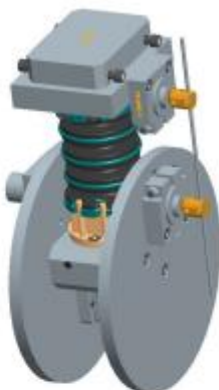
Figure 51 Q10 Neck Certification Setup for Frontal Extension Test, View Looking from Front in Drop Position
